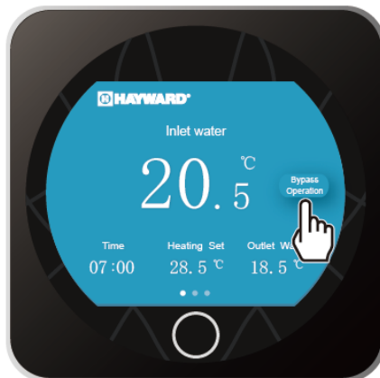
Activate Bypass Operation
