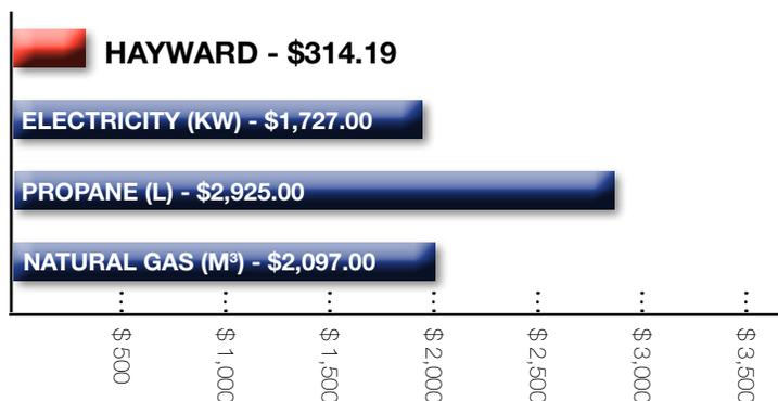
\*Based on HP65BEE1 heat pump with an in-ground pool 14' x 28' with an air temperature of 80° F, humidity 62% and a water temperature of 80° F in Quebec. Comparison based on a cost of \$ 0.065 per kWh of electricity.
