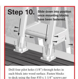
mounting block. Drill three holes through each
