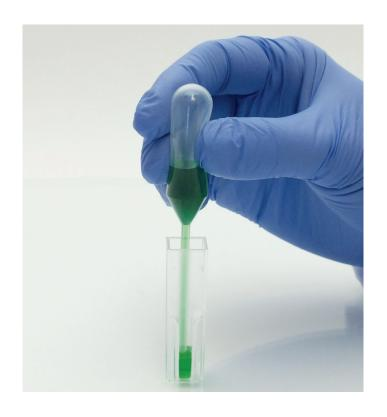
In chromatography for industrial research and testing the Large Bulb Micro is great for sample preparation. It is also good for water sampling applications in the field, or as a portable ampoule for reagent handling and storage.
