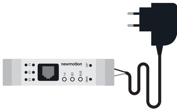
**Note:** Polarity is important! 1 of the 2 power adapter wires has a broken white stripe. This wire is the power adapter GND and should therefore be connected to the GND pin (right) on the module. The other wire is the +5 Volts and should be connected to the +5V pin (left) on the module. The middle pin is not used.
