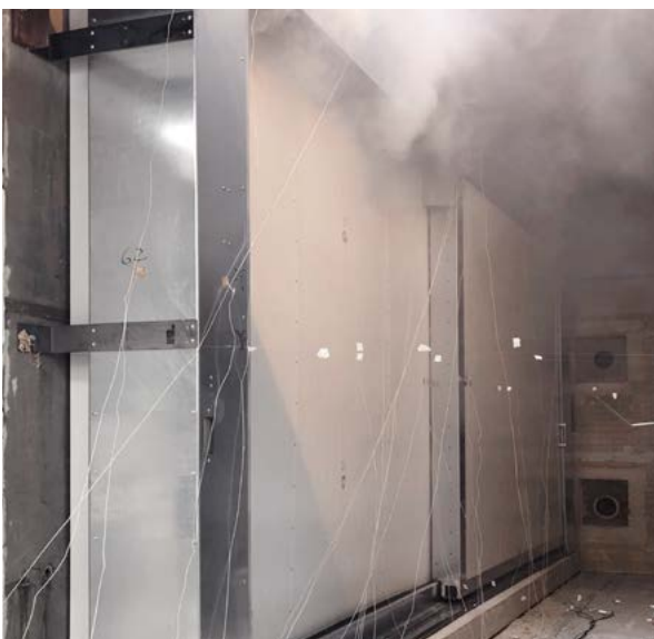
RFP SD with sliding doors during fire test. Smoke is emitted from cracks but there is no flashback. In the next few moments, the protective mechanism will take effect and suppress the smoke.
