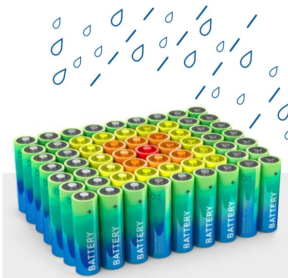
Schematic diagram of a larger, damaged battery module with water cooling by sprinkler system.
