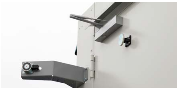
Automatic door closing and hold-open system with upper door closer. The door is held open by an electromagnet as a counter-support. To close the door, the power to the retaining magnet is cut.
