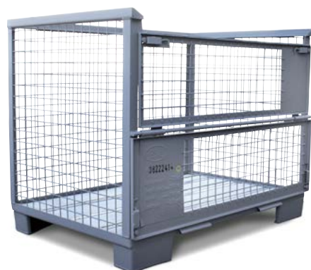
EURO skeleton box acc. to UIC 435-3, with 2 flaps, grey, front wall with 2 flaps and 2 labelling panels, outer dimensions W x D x H (mm): 1240 x 835 x 970, order number 129-203-T1
