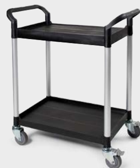
General purpose trolley, tubes made of brushed aluminium, 2 tiers, W x D x H [mm]: 480 x 850 x 950, overall load capacity [kg]: 160, order number 180-037-T1
