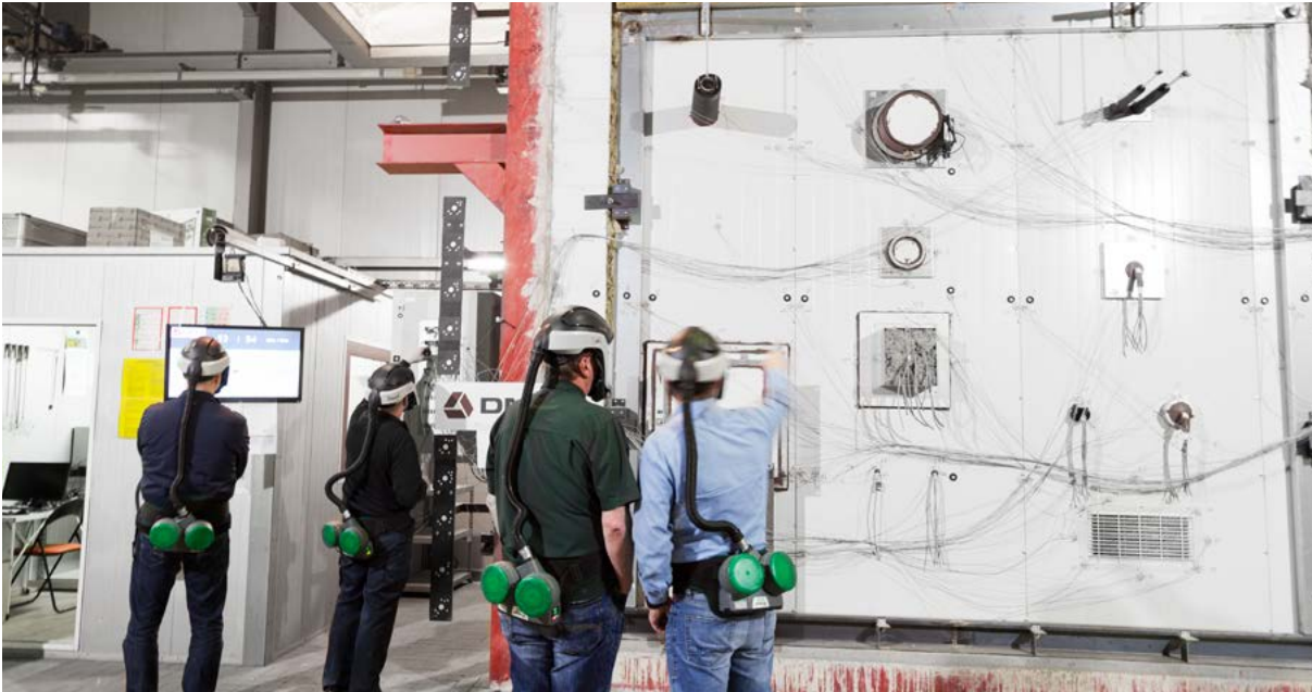
Successful performance of a fire test for different types of fire seals (cable and pipe break-through points).
