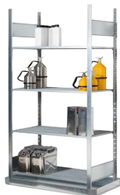
Hazmat shelving model GRB 1060, with steel sump and 4 grid shelves, external dimensions W x D x H (mm): 1156 x 726 x 2000, order number 199-716-V1
