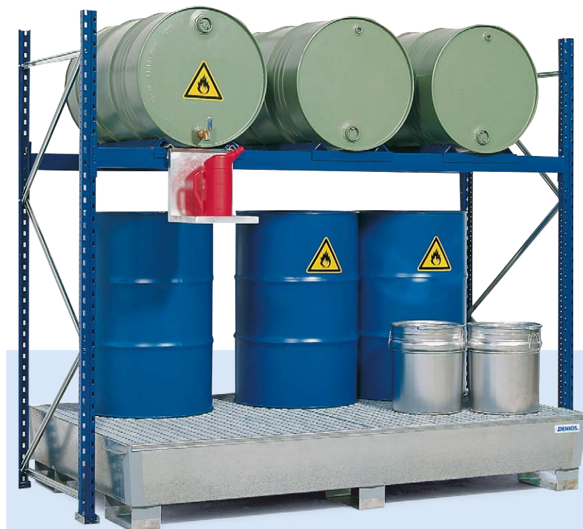
Drum Rack for 3 drums horizontally and 6 vertically on gratings (dispensing shelf sold separately) Order no. K34-1109-U2
