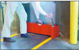
Within seconds the doorway is secured against flowing liquids.
