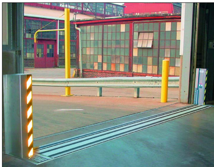
Pop-Up Automatic Doorway Spill Barriers quickly seal off a room, preventing any spill from contaminating other parts of your plant. The ADSB operates without any power assist and lays flat until triggered by a spill.
