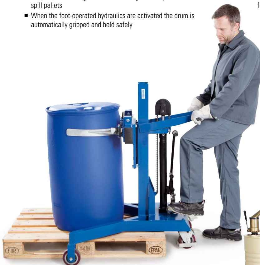
For 200 litre steel drums and 220 litre plastic drums, load capacity 300 kg, order number 201-867-H1
