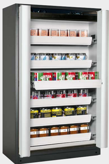
Select hazardous substances cabinet with folding doors. The slide-out spill sumps make it easy to safely see what hazardous substances are stored in the cabinet. Order no. 233-806-N1
