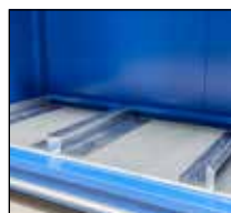
"Pushback trolley" - system for "Last-In-First-Out" loading
