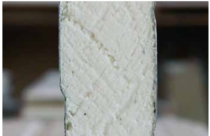
Section through the PUR panel wall insulation (construction material class B). This material has better insulation properties and is flame-retardant.
