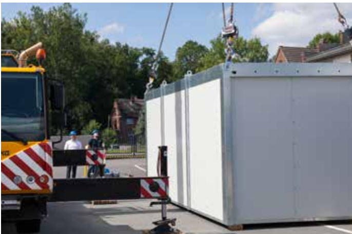
The technical room system loaded with weights is lifted
