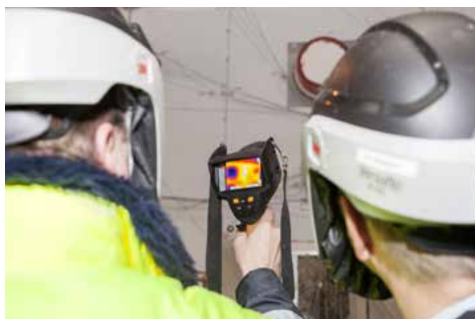
Checking fire tests with thermography
