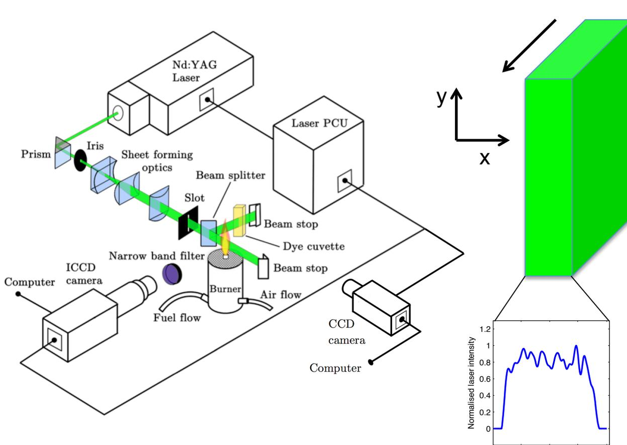
Laser: Litron Nd:YAG laser, 150mJ @ 532nm, 10 H<sub>2</sub>
