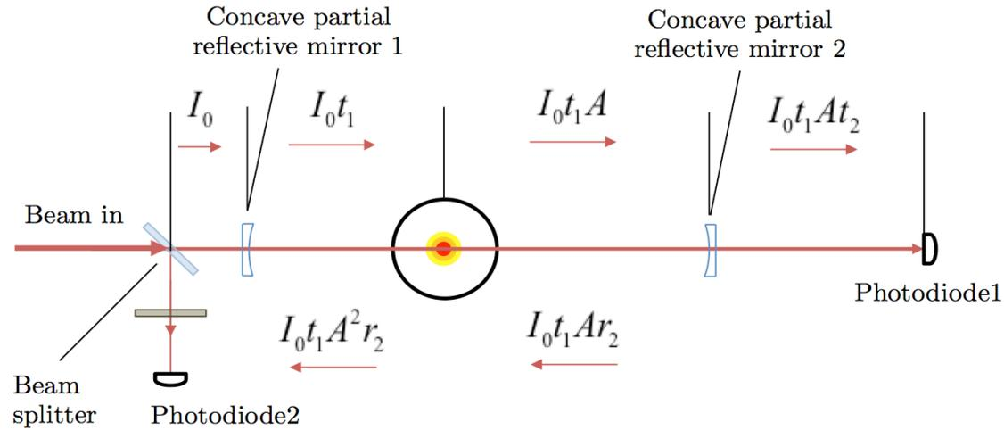
$$\left\{ \begin{array}{l} P_t = g(\mathbf{V}, C) \\ P_t = \frac{I_t}{I_i} = \frac{A(1-R)}{1-A^2R} \\ P_0 = -\ln A = \int_{-\infty}^{+\infty} K_{ext} dx \\ K_{ext} = \frac{6\pi E(m)}{\lambda} f_v \end{array} \right.$$
