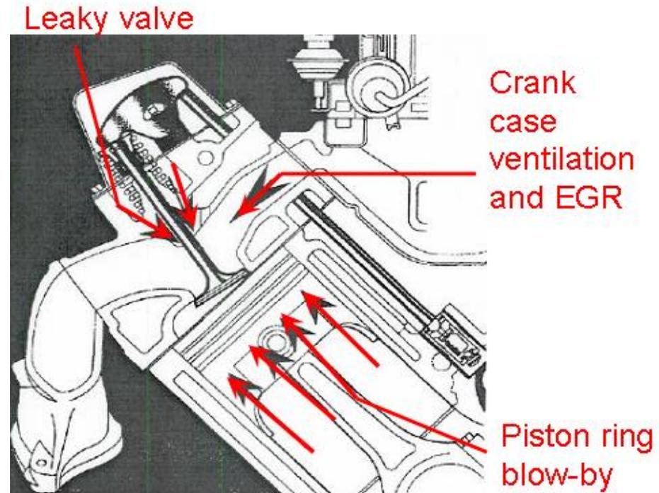
Diagram of lube oil pathways on a typical engine (modified from Hill and Systasma, 1991)
