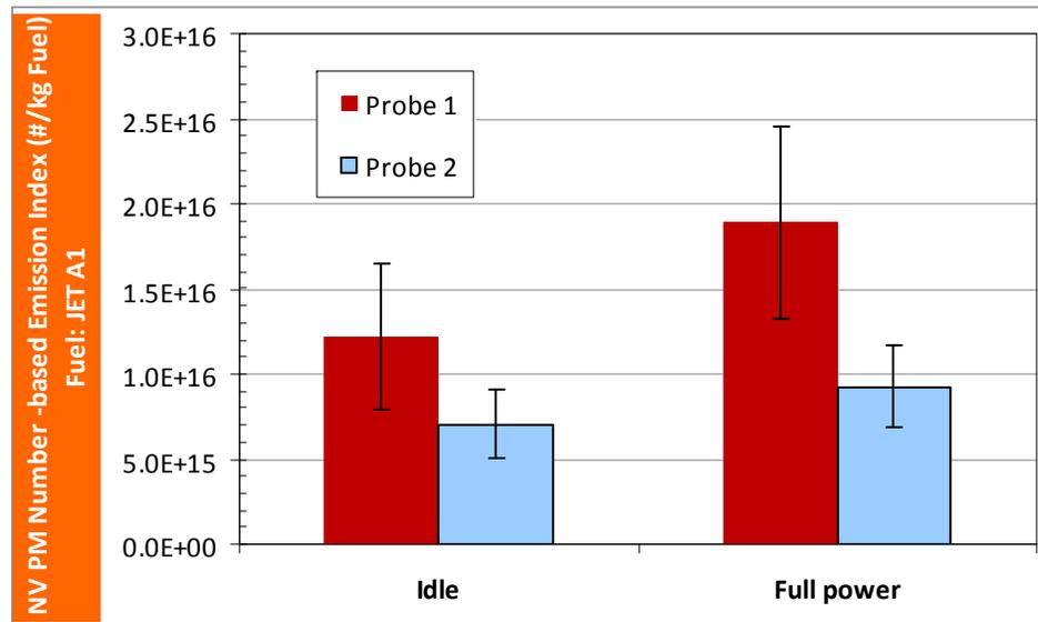
Probe 1: Dilution at probe tip
