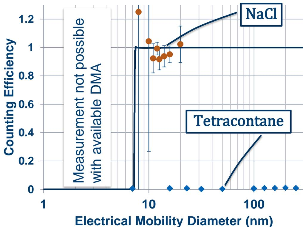
— Predicted Counting Efficiency for Solid Particles
