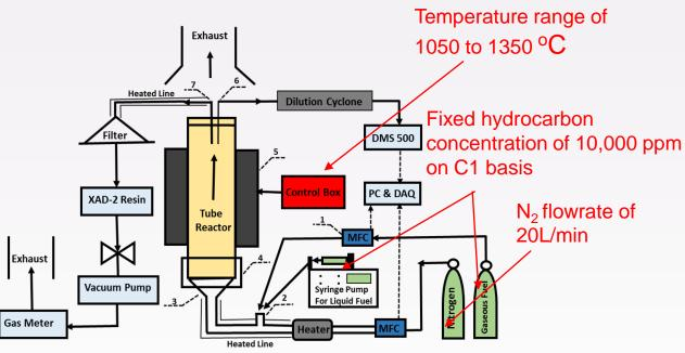
Schematics of the experimental set-up: 1) mass flow controller (MFC) 2) vaporiser 3) static mixer 4) circulating cooling water 5) tube furnace 6) DMS 500 sampling probe 7) soot sampling probe
