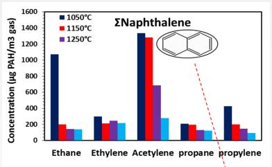
Naphthalene was the most abundant PAH found during the pyrolysis of a triplebonded acetylene
