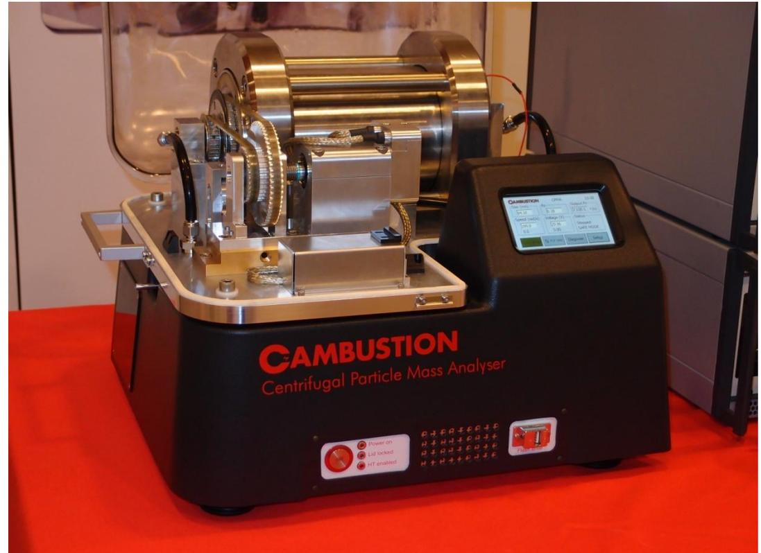
200 l × 120 ø mm classifier with 1 mm gap; 0.1–1000 V; 500–12,000 rpm
