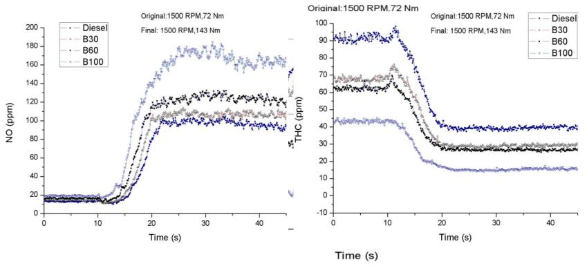
•The initial decrease of NO was small compared with previous test. B100 Produced the highest NO to initial ratio became smaller when highest
