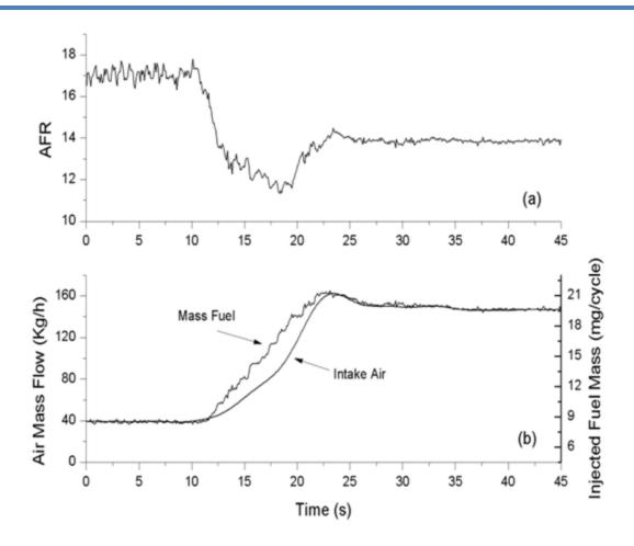
Diesel AFR (a) and Intake Air with Fuel Injection (b) for Mode 1-3 (750RPM, 36Nm-1500RPM, 143Nm in12s)
