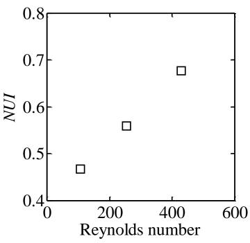
The through-wall velocity profile becomes <u>less uniform</u> as the inlet gas flow rate increases
