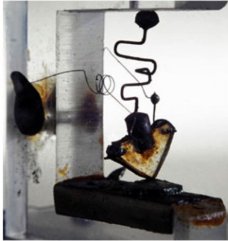
First build transistor, 1948 (Germanium based)
