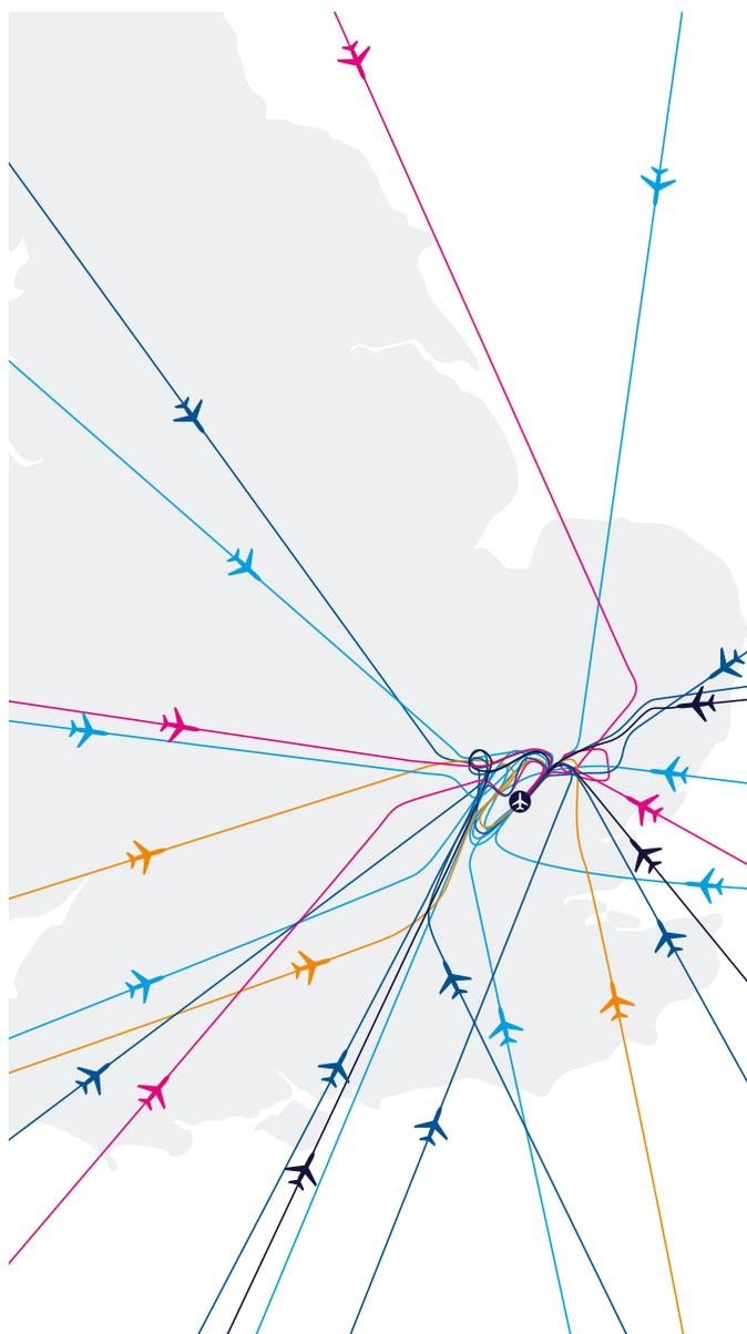
Unlike departing aircraft there are no fixed flight paths for arriving aircraft until they are established on the Instrument Landing System (ILS), also known as the 'final approach'. There are also no fixed noise limits or heights.
