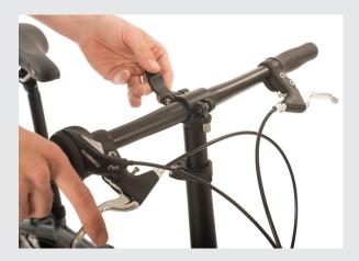
It is possible to rotate the handlebar into the desired position by pulling up the top clamp, re-positioning and pressing it fully down. Recommended riding position is with the brake levers pointing down 15° from the horizontal.
