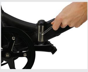
**Clamp adjustment** If the clamp feels loose and is too easy to push down the tightness can be adjusted by tightening the screw on the opposite side of the frame using a 6mm Allen and turning clockwise.
