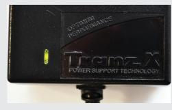
The green light indicates that the battery is fully charged.
