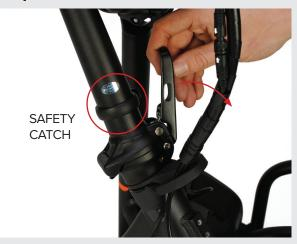
Pull down the lever & fold handlebar down
