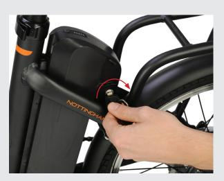
Insert the key and turn clockwise and slide the battery out. To fit, slide back in and ensure the bottom fits into the controller.
