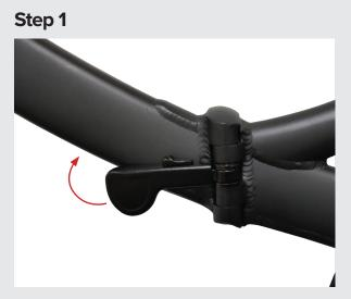
To lock push down the lever firmly against the frame
