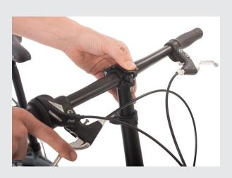
**Important: Before each ride** Always check that the handlebar is fully tightened and cannot rotate. The tightness of the clamp can be adjusted with the clamp screw underneath.
