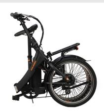
To finish folding operation loosen seat post clamp & push the seat post down to the floor
