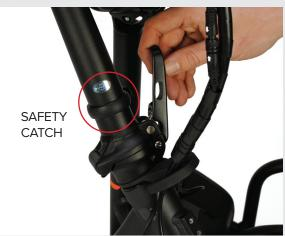
Fold handlebar by rotating the safety catch Important: When folding into the riding position ensure that the safety catch fully engages into the slot in the clamp lever
