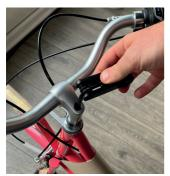
Make sure the forks are facing forward then, using the 6mm Allen key, loosen the bolt on the top of the stem so that the stem will rotate side to side.
