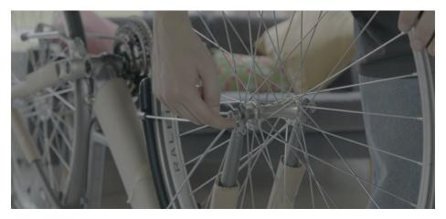
Tighten nuts by hand and then use the pedal spanner (or any 15mm spanner), to tighten them off.
