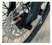
Hand tighten the skewer nut until you can fold the lever up with resistance. You should feel significant resistance when folding and unfolding the lever.
