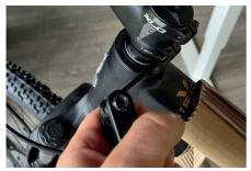
Align handlebar stem with the front wheel and tighten the two side bolts below.
