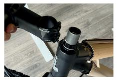
Make sure the forks are facing forward then insert the handlebars into the headtube with the brakes at the front.
