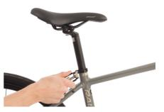
You must not pull the seat post out further than the limit mark. This must not be visible.
