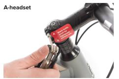
Using the multi tool provided, tighten the 2 stem clamp bolts shown as A and B in the above photo. Max 6Nm unless stated otherwise on the component.
