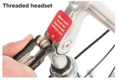
Using the multi tool provided, tighten the bolt in the top of the stem (shown as C in the above photo). The bolt may be under a rubber bung. Max. 15Nm unless stated otherwise on the component.
