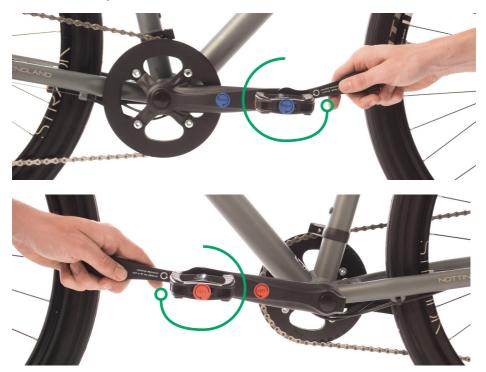
Once the pedals are attached and tightened the RIGHT and LEFT stickers can be removed.
