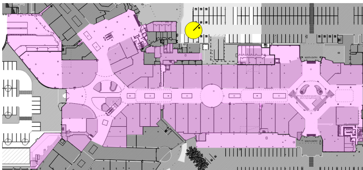
Figure 31: Extent of the EWIS system upgrade – Ground Floor.
