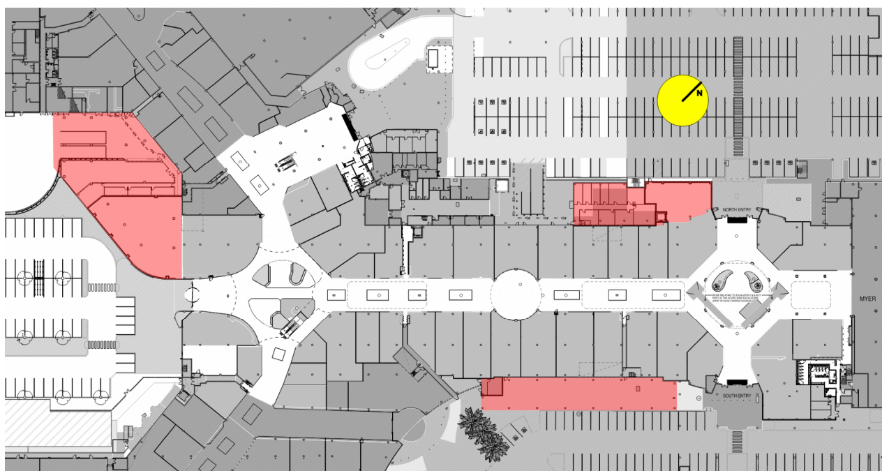
Figure 44: Ground Floor areas where load bearing structure has performance-based reduced FRL
