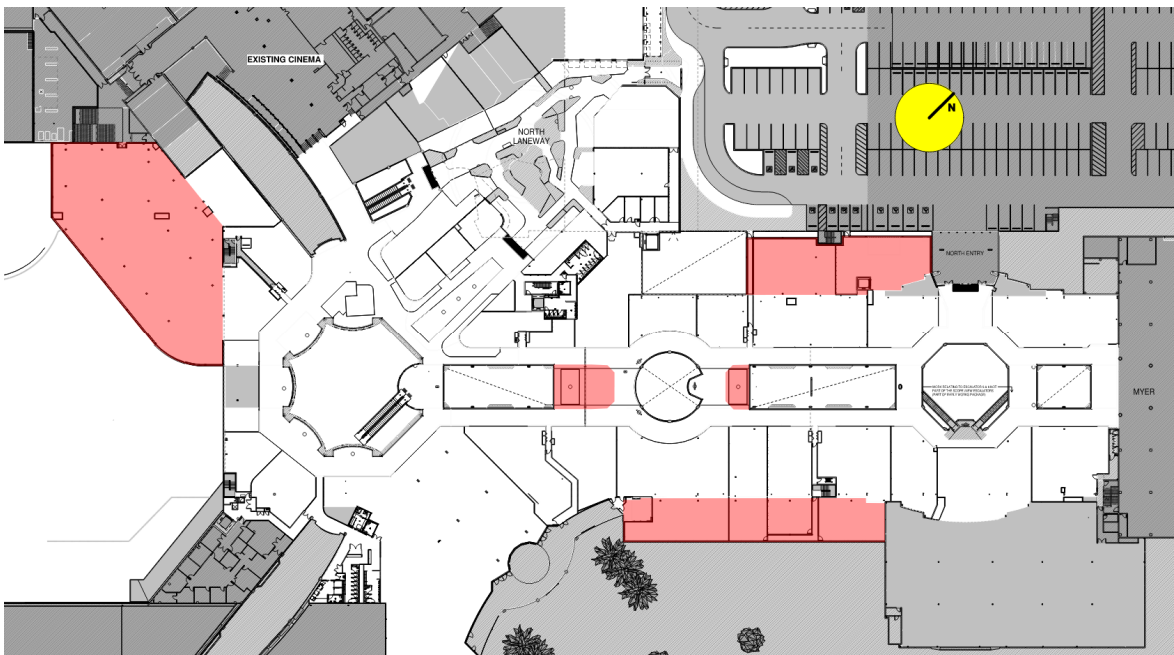
Figure 10: First Floor areas where load bearing structure has performance-based reduced FRL
