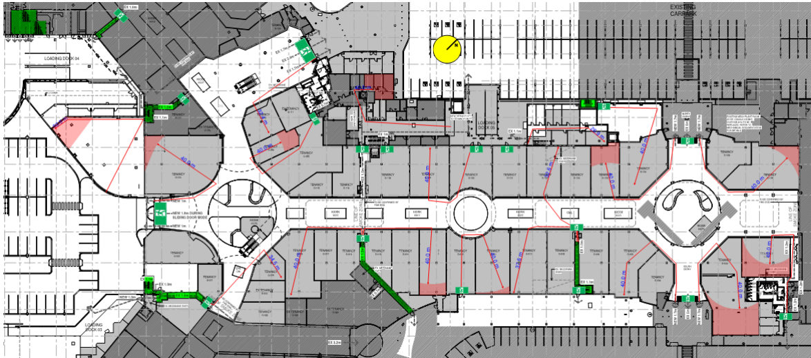
Figure 49: Travel distances to the nearest of alternative exits on Ground Floor
