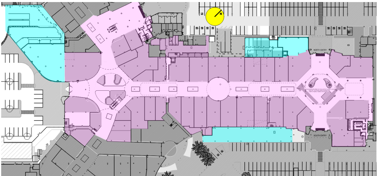
Figure 59: Areas where fire hose reels are omitted on Ground Floor
