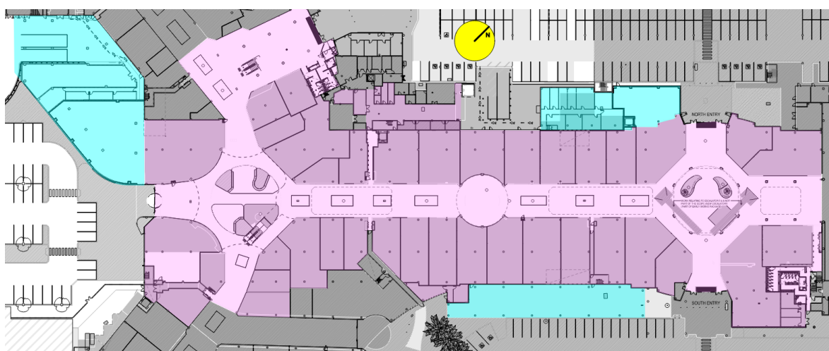
Figure 16: Areas on Ground Floor where hose reels may be omitted
