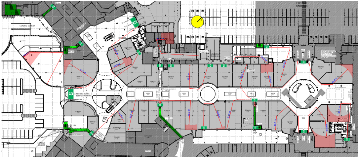
Figure 52: Travel distances to the nearest of alternative exits on Ground Floor
