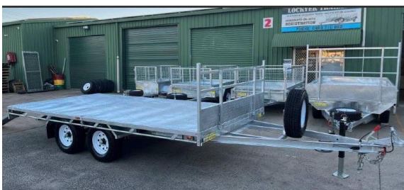
Figure 6 Example of trailer that can be used to transport flat lay glass stillage.
