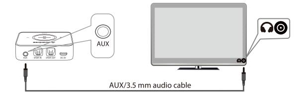
After connecting your audio cable you should be able to hear sound from your headphones; if not: 1) Ensure the AUX/SPDIF (Optical) switch on the TC417 is set to the "AUX" position.
