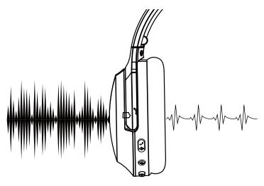
After power ON, slide ANC switch to "ANC" to activate the ANC function. The ANC LED light will turn GREEN.
