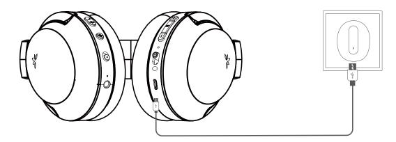
When the LED starts blinking RED once every 10s or indicator solid RED, or when you hear "beep" / prompts sound, you should recharge your headphones. Please plug it into a USB wall charger (DC 5V / 0.5-2A) or a powered USB port via the micro USB cable that we provided.
