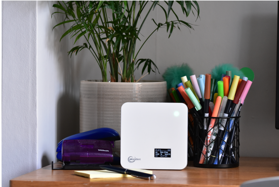
Figure 1. Indoor air quality sensors deployed by the Schools' Air Quality Monitoring for Health and Education program in the United Kingdom. Low-cost sensors measuring carbon dioxide, total volatile organic compounds, particulate matter, temperature, and relative humidity were deployed in over 1,300 schools.
