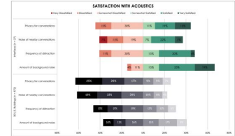
Acoustic satisfaction at Interface Base Camp compared to a benchmark sample of 30 U.S. offices. Responses were on a 7-point Likert scale ranging from very dissatisfied to very satisfied. Percentage of overall responses are not included in the graph.
