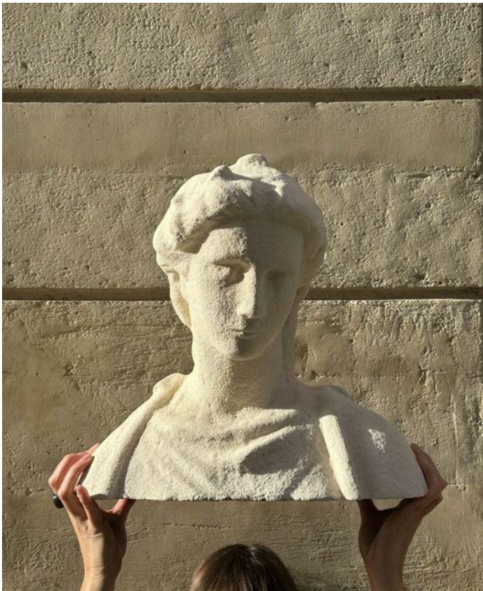
BUST PROTOTYPE Expanded cork and rammed earth
