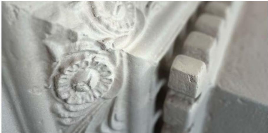
CORNICE PROTOTYPE Expanded cork
