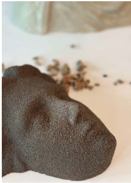
HEAD PROTOTYPE Lime and cork
