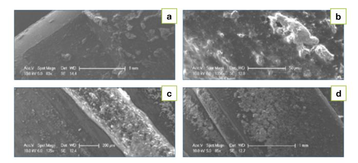
Images: Examples of contaminants that were found on decontaminated surgical devices. All the figures described previously were from before decontamination. The organic contaminant in picture (a) is shown at 83x magnification. The contaminant encased in lubricant in picture (b) is shown at 1356x magnification. The contaminant in picture (c) is shown at 175 x magnification and the sulphur-based contaminant in picture (d) is shown at 85x magnification.
