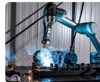
**Welding:** Agricultural machinery manufacturers often operate MIG welding cells, however, there is a shortage of reliable, skilled labour in this area. Many OEM manufacturers are turning to automation for cell welding so that a single, un-skilled operator is able to manage several cells simultaneously without reducing the quality of the output.
