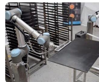
**Tray Handling:** The stacking of trays on the end of a line or the feeding of trays into a washer is a monotonous and repeatable process that can be easily automated. A robot can be programmed to pick from racks or stack into racks, freeing up your team to engage in greater value-added activities.
