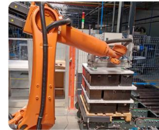
**Palletising:** Loading products onto pallets from the end of a production line is ideal for robots. This is probably the most common use for robots in the food industry right now and one of the easiest to implement. A perfect example of a repeatable and predictable job for a robot to do 24/7.
