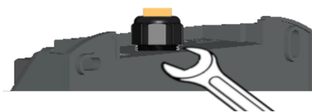
Fig. 6-15: Tighten the cable gland from the back
