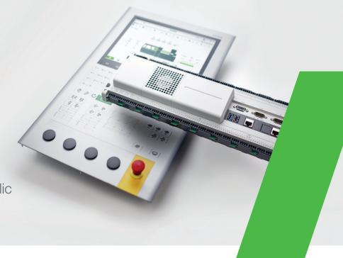
KePlast i1100 combines an outstanding and user-friendly operation with established keyboards and complete performance control for the highest productivity – perfectly designed for hydraulic standard injection molding machines. The Linux-based software platform is future-proof and enables Industry 4.0 requirements, communication protocol, and interface standards, such as OPC UA & EUROMAP 77.
