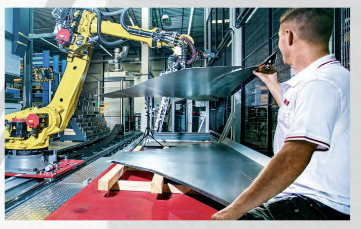
At the agricultural machinery manufacturer RAUCH, the KeMes angle measurement device is also used to check angles by hand. Especially in the robot bending cell, the new protractor made the process of manual follow-up inspection much faster and easier.
