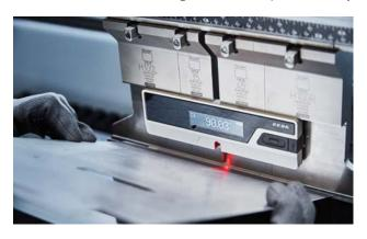
resulting in considerable time savings. In addition, a specially designed function enables continuous measurement along the entire workpiece.
