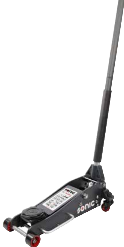
#48031 Aluminum + steel jack, 1,5 ton • Maximum lifting capacity: 1500kg • Minimum lift height: 88mm • Maximum lift height: 360mm • Total length: 484mm • Diameter pick-up dish: 108mm
