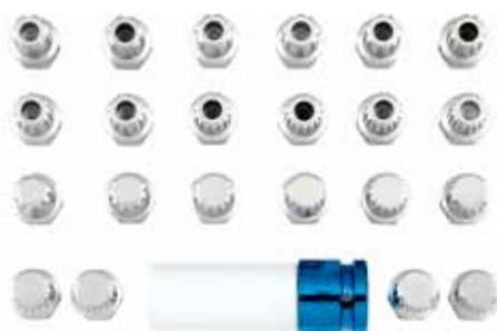
#829006 Wheel nut key set - suitable for Audi 22-pcs Set complete including 21mm adaptor with 1/2 "square drive. This kit is designed for the removal of locking bolts when the customer has forgotten to provide the adaptor with the car. This is happening very often when the vehicle is brought to maintenance and/or repair. Suitable for OEM T40073.
