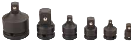
#300605 Impact adaptor set 6-pcs 1/4"(F)x3/8"(M), 3/8"(F)x1/4"(M), 3/8"(F)x1/2"(M), 1/2"(F)x3/8"(M), 1/2"(F)x3/4"(M), 3/4"(F)x1/2"(M)
