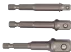
#100301 Adaptors for drills, 1/4", 3-pcs - 6.3 + 10 + 12.5mm square (1/4"+3/8"+1/2") with ball - 6.3mm (1/4") hex drive, for use of standard spanner sockets in chucks
