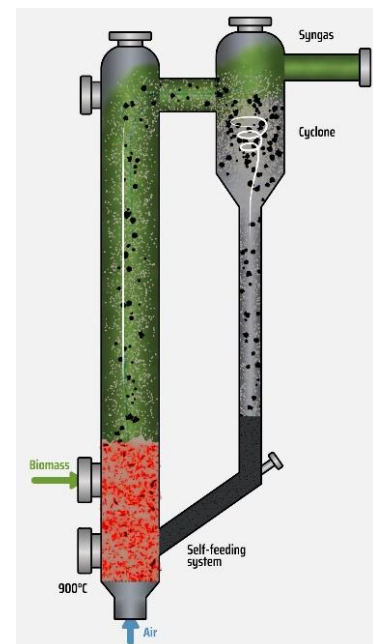
Figure 4: Sketch of the HFB gasifier. To produce industrial gases, oxygen is used instead of air, as the aim is to minimize the amount of nitrogen gas in the process.
