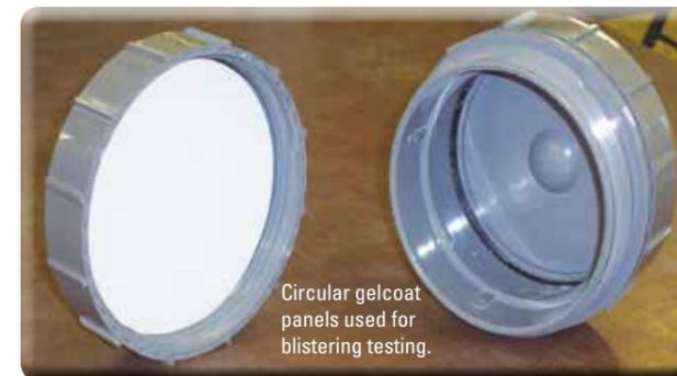
Circular gelcoat panels used for blistering testing.
