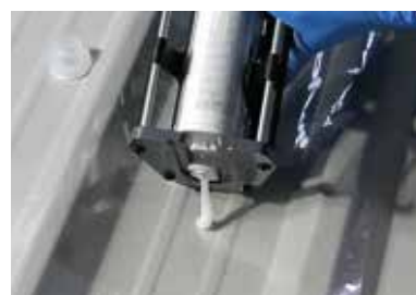
Figure 4 Dispense material to level plungers.
