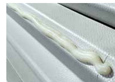
Figure 6 Apply adhesive to bond area.
