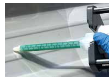
Figure 5 Attaching the mix head.
