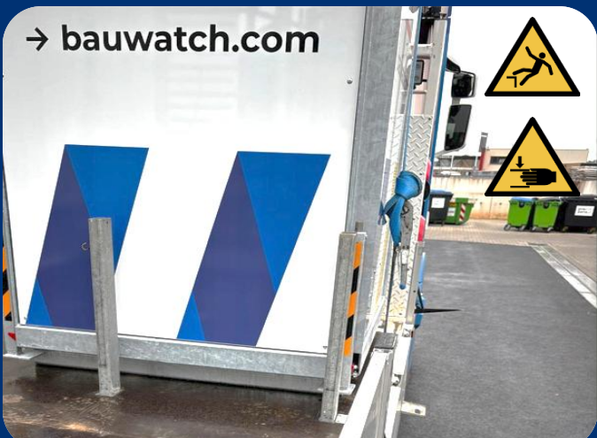
4. Position the stakes to prevent sliding.
