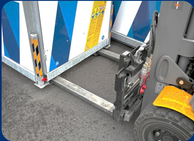
1. Always use the sleeves for the forks of the forklift truck.
