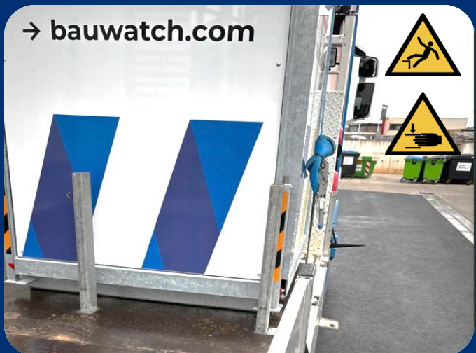
4. Position the stakes to prevent sliding.
