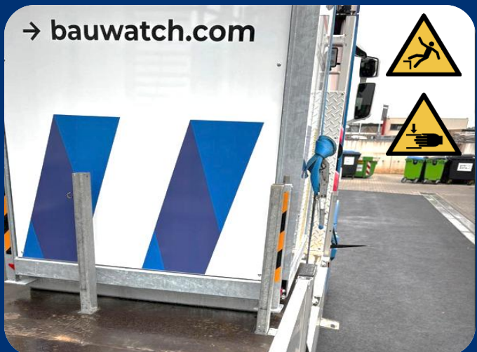
4. Position the stakes to prevent sliding.
