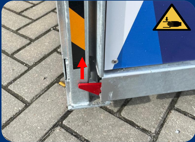
1. Turn the red lock upwards to pull out the support legs.
