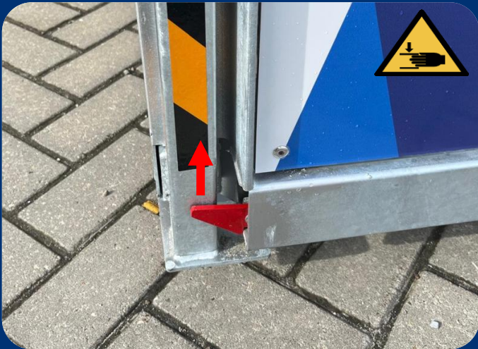
2. Turn the red lock upwards to pull out the support legs.
