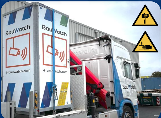
5. Secure the tower using a lashing strap, taking care to ensure that the frame does not bend.
