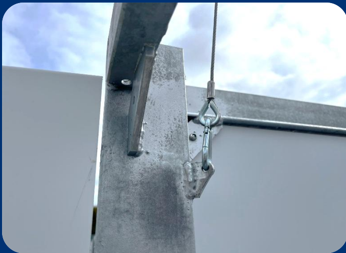
6. Before the mast is fully extended, check the hooks again to ensure they are still secure.
