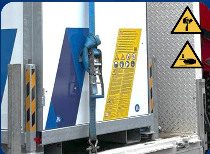
6. Secure the excess length of the lashing strap.
